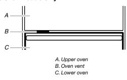
The oven vent(s) should not be blocked or covered since they allow the release of hot air and moisture from the oven. Blocking or covering vents will cause poor air circulation, affecting cooking and cleaning results. Do not set plastics, paper or other items that could melt or burn near the oven vent(s).
