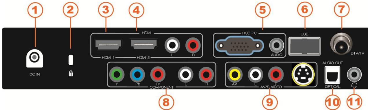
1. **DC IN**—Connect the included AC/DC power supply here. Connect the other end to a wall outlet.
