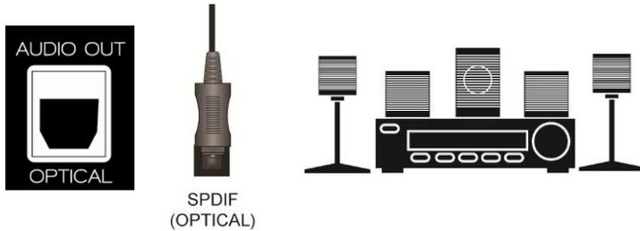
If your sound system has a SPDIF (optical) digital audio input you can connect it to the **OPTICAL** digital audio out on the back of your HDTV. This is active when receiving audio with the content being viewed no matter which input is being used.
