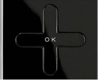
**Up, Down, Left or Right navigation buttons** — Press to navigate open menus, adjust other TV settings such as Brightness and Contrast, or turn menu options On and Off.
