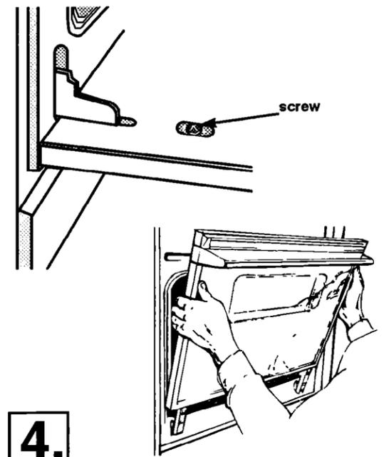
**4.** Close lower oven door to the broil position. Grasp the sides of the oven door and pull the door up and out of the hinge slots to remove. Set door aside.
