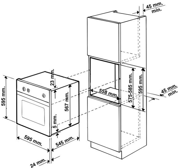
In order to ensure adequate ventilation, the back panel of the cabinet unit must be removed. Installing the oven so that it rests on two strips of wood is preferable. If the oven rests on a continuous, flat surface, there must be an aperture of at least 45 x 560 mm.
