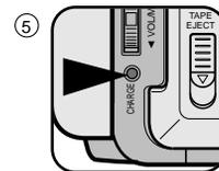
5. When the battery is fully charged, disconnect the battery pack and the AC Power adapter from the camcorder.
