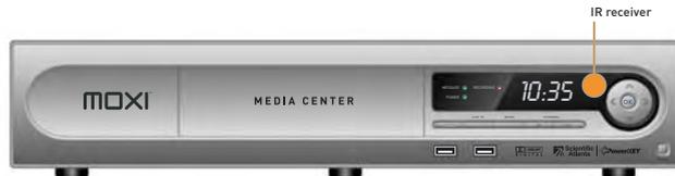
Figure 40: Infrared receiver on the media center front panel
