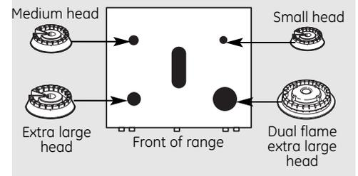
Make sure the slot (on front left, back right and back left heads) and the hole (front right head) in the burner head is positioned over the electrode.
