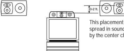
This placement provides a wide spread in sound, supplemented by the center channel speaker.
