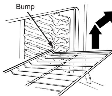
To replace, place the shelf on the shelf support with the stop-locks (curved extension of shelf) facing up and toward the rear of the oven. Tilt up the front and push the shelf toward the back of the oven until it goes past the bump on the shelf support. Then lower the front of the shelf and push it all the way back.
