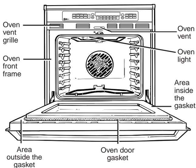
3. Clean spatters or soil on the oven front frame and the oven door **outside the gasket** with a dampened cloth. The oven front frame and the oven door outside the gasket do not get cleaned by the self-clean cycle. On these areas, use detergent and hot water or a soap-filled steel wool pad. Rinse well with a vinegar and water solution. This will help prevent a brown residue from forming when the oven is heated. Buff these areas with a dry cloth. Do not clean the gasket.
