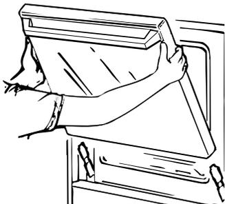
**To remove the door,** open it a few inches to the special stop position that will hold the door open. Grasp firmly on each side and lift the door straight up and off the hinges.
