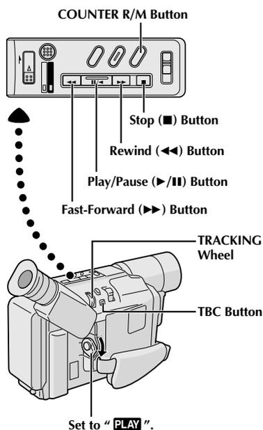
**Tracking:** Eliminates noise bars that appear on-screen during playback. Factory-preset is Auto Tracking. To activate Manual Tracking:
