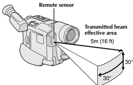
When using the remote control, be sure to point it at the remote sensor. The illustration shows the approximate transmitted beam effective area for indoor use.
