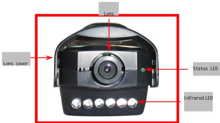
Figure 2. CAM77IP Network Camera Front View
