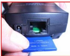
Figure 6. Insertion of SD memory storage card
