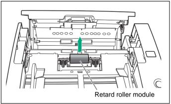
5 Install the new retard roller module by matching the groove of its shaft with the groove of the metal holder. Make sure that both ends of the shaft
