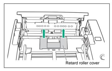
**4** Remove the retard roller module in the direction of the arrow.
