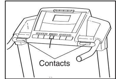
**stand on the foot rails** and hold the metal contacts—**avoid moving your hands**. When your pulse is detected, your heart rate will appear on the screen. **For the most accurate heart rate reading, continue to hold the contacts for about 15 seconds.**
