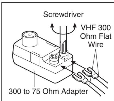
2. Push the 300 ohm to 75 ohm adapter onto the 75 ohm antenna terminal on the treadmill frame near the power cord.
