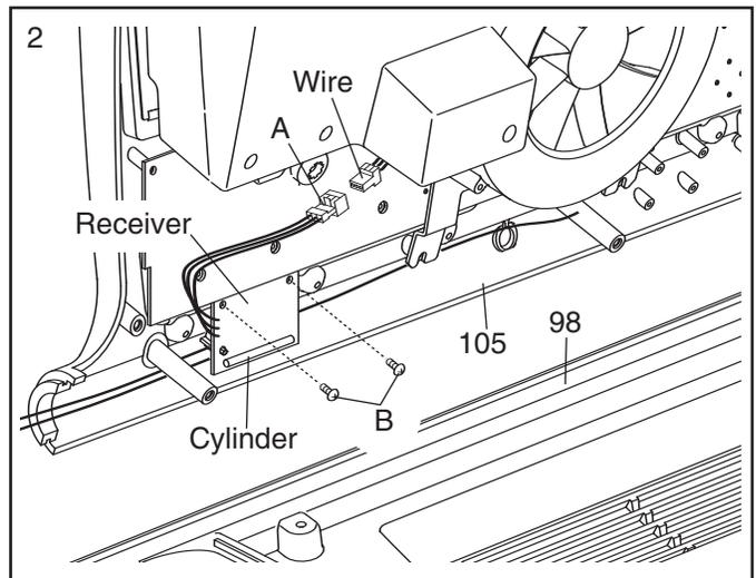
3. **Make sure that no wires are pinched.** See drawing 1. Reattach the Console (105) to the Console Base (98) with the 3/4" Screws (7). Discard the other wires included with the receiver.
