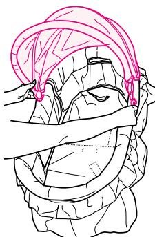
Insert canopy mounts into slots on each side of bassinet frame.
