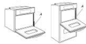
Single Oven A. Model/serial number plate Double Oven A. Model/serial number plate
