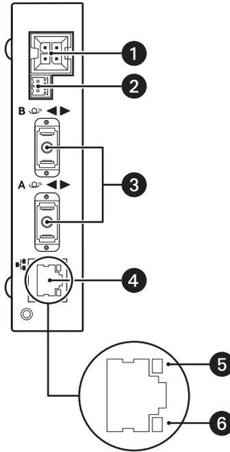
**Figure 4.** Rear Panel of FX82012 Module (SC Fiber Connectors Shown)
