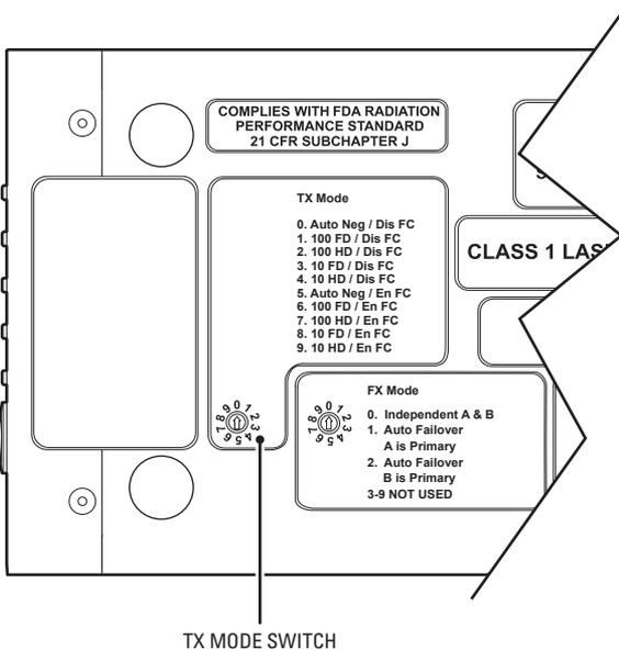
**Figure 5.** TX Mode Switch for 10BASE-T/100BASE-TX Port
