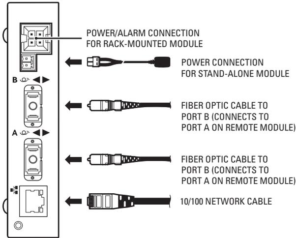
**Figure 8.** FX82012 Connections (SC Fiber Connectors Shown)
