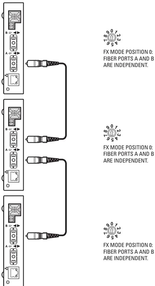
**Figure 10.** Fiber Port Connections in Sample Drop-and-Repeat Application
