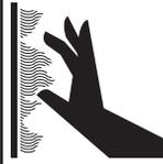
METAL PARTS OF THIS EQUIPMENT BECOME EXTREMELY HOT WHEN IN OPERATION. TO AVOID BURNS, ALWAYS USE HAND PROTECTION WHEN OPERATING THIS APPLIANCE.
