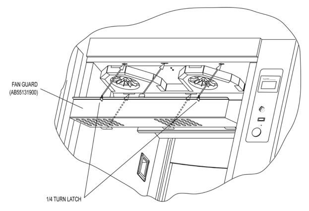
b. Pull Circulation Bottom out of oven then unscrew (clockwise) the wing nut on each Blower Fan to remove the fan blades.
