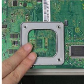
7. The heatsink paste helps to enhance heat dissipation of the CPU. Before installing the cooler set (fan & heatsink bundled), make sure that you detach the shield of the heatsink paste under the cooler set.
