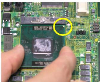
4. On the front end of the CPU socket is a locking mechanism designed in the form of a screw head. Make sure that you actuate or deactivate this mechanism with a screwdriver before and after installing the CPU.
