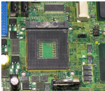
2. Place the CPU on top of the socket. Make sure to align the gold arrow on the CPU with the arrow key on the socket.
