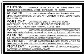
This label is located on the Laser protective housing inside the enclosure.
