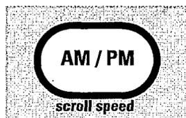
The scroll speed of the display can be changed. Press and hold the AM/PM pad about 3 seconds to bring up the display. Select 1-5 for slow to fast scroll speed.
