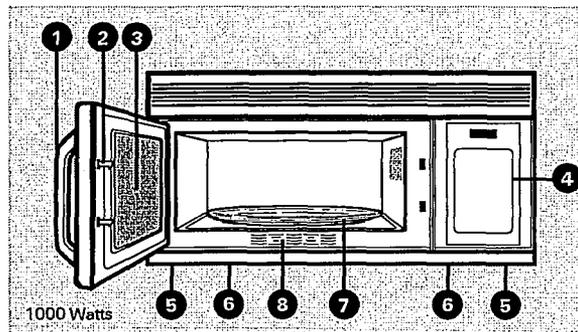
**1 Door Handle.** Pull to open the door. The door must be securely latched for the microwave to operate.
