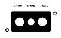
The J2-360.2's "+12VDC" and "Ground" connections are designed to accept 4 AWG power wire. 4 AWG is a minimum power wire size for this amplifier.
