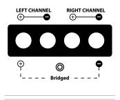
J2-360.2 is designed to deliver power into speaker loads equal to or greater than 2 ohms per channel when using a "stereo" configuration and speaker loads equal to or greater than 4 ohms when using a "bridged" configuration.
