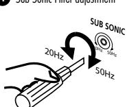
**(Eng)** Adjust the frequency of departure of the Subsonic filter from 20 to 50Hz in agreement to the connected loudspeaker.
