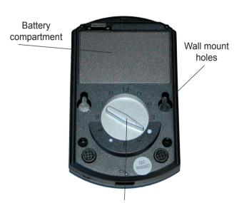
12 Position rotary switch to match the connections in your handset
