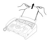
Open the top cover by lifting the lever on the right side of the top cover.
