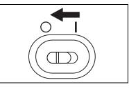
Press the battery chamber cover button on the side of the instrument and slide the cover downward to open it.
