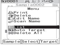
3 To return to the <Sample> screen, press the [MENU] button while the <Menu> screen is displayed.
