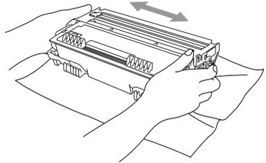
**!** To prevent damage to the drum, do not expose it to light for longer than a few minutes.
