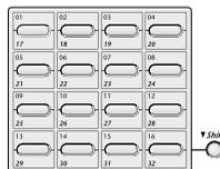
*One Touch keys are the 16 keys (numbers 01–32) located on the left side of the control panel.*
