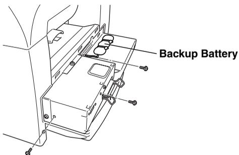
**4** Disconnect the connector from the backup battery.
