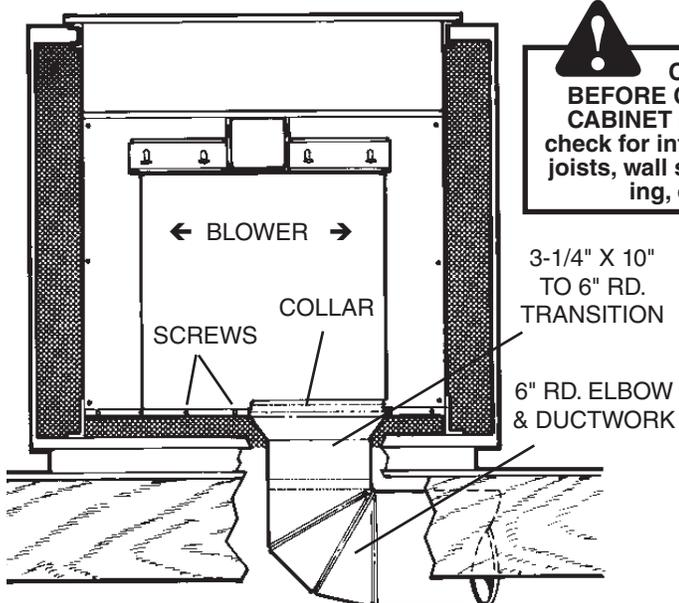
1. Cut hole in cabinet as well as holes in wall or floor as necessary.
