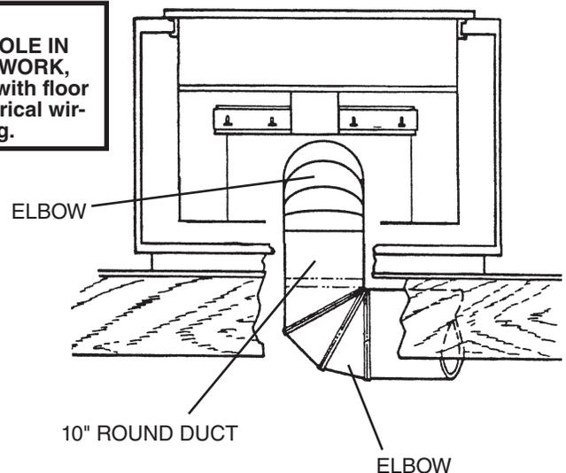
1. Cut hole in cabinet as well as holes in wall or floor as necessary.
