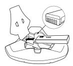
⇒ Connect to a DECT system (see page 11), a mobile phone or a computer as illustrated. (An optional phone cable is required for connection to mobile phones.)
