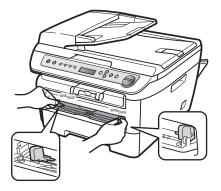
4 Using both hands, put one sheet of paper or one envelope in the manual feed slot until the front edge of the paper or envelope touches the paper feed roller. When you feel the machine pull in the paper, let go.
