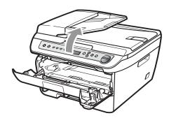
Use both hands to carefully pull the jammed paper up and out of the output tray opening.
