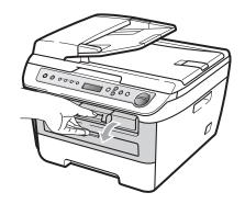
Slowly take out the drum unit and toner cartridge assembly. The jammed paper will be pulled out with the toner cartridge and drum unit assembly.
