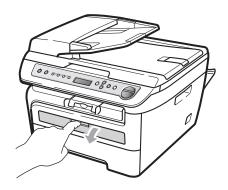
3 Using both hands, slide the manual feed slot paper guides to the width of the paper that you are going to use.
