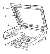
(DCP-7040 only) In the ADF unit, clean the white bar (1) and the scanner glass strip (2) underneath it with a soft lint-free cloth moistened with water.
