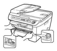
4 Using both hands, put one sheet of paper in the manual feed slot until the front edge of the paper or transparency touches the paper feed roller. When you feel the machine pull in the paper, let go.
