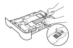
3 Put paper in the tray, and make sure that the paper is below the maximum paper mark (1). The side to be printed on must be face down.
