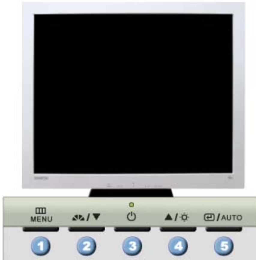
1. **Menu button** [☰] Use this button for open the on-screen menu and exits from the menu screen or closes screen adjustment menu.
