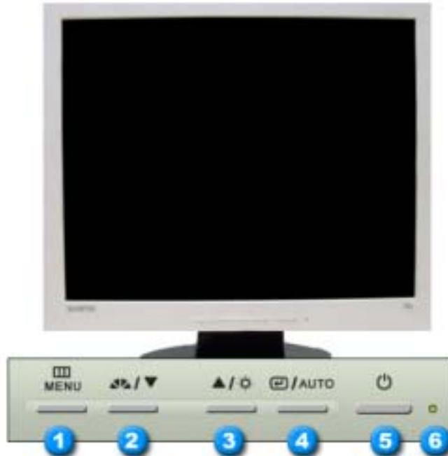
1. **Menu button** [MENU] Use this button for open the on-screen menu and exits from the menu screen or closes screen adjustment menu.
