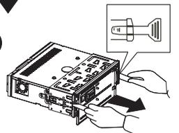
5. Pulling the levers makes it possible to remove the unit from the dashboard .
