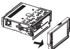
2. Remove the control panel .
