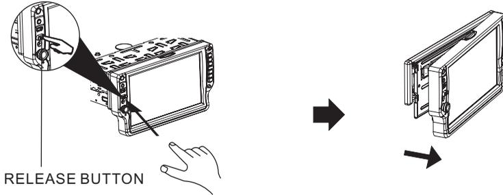
2). Pull-off the front panel and keep the front panel into the case .
