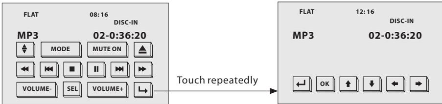
In stop mode, touch the ↑ / ↓ / ← / → sections on touch screen (or Use ▲ / ▼ / ► / ◀ on the remote control ) to select the item or folder, then touch the “OK” range (or press **ENTER** button on the remote control ) to confirm.
