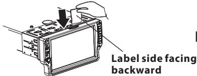
Insert the memory card into slot with label side facing backward .
