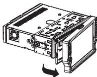
1. Press the **REL** button to release the front panel .
