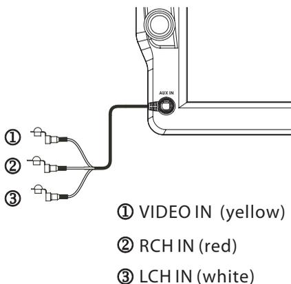
1) Please connect the external device with stereo jack plug the Aux in socket .
