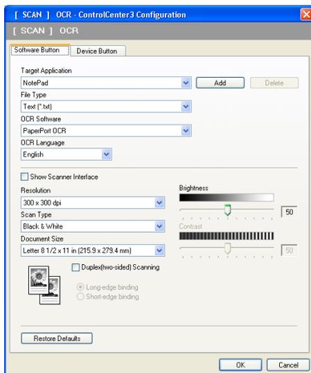
To change the word processing application, choose the destination word processing application from the **Target Application** drop-down list. You can add an application to the list by clicking the **Add** button. To delete an application, click the **Delete** button in the **Software Button** tab.
