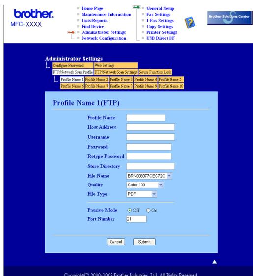
You can set Passive Mode to OFF or ON depending on your FTP server and network firewall configuration. By default this setting is OFF. You can also change the port number used to access the FTP server. The default for this setting is port 21. In most cases these two settings can remain as default.
