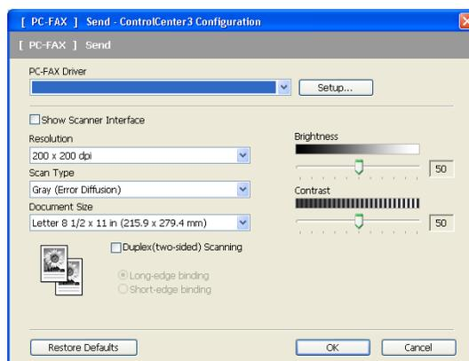
If you want to scan a duplex document, check **Duplex(two-sided) Scanning** and choose **Long-edge binding** or **Short-edge binding**. (Not available for the DCP-8080DN and MFC-8480DN)
