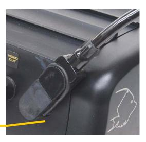
6 pin connector mated and secured with retainer strap
