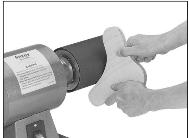
Figure 1. Typical drum sanding operation.
