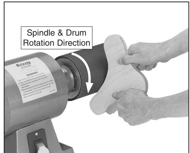
Figure 15. Typical drum sanding operation.
