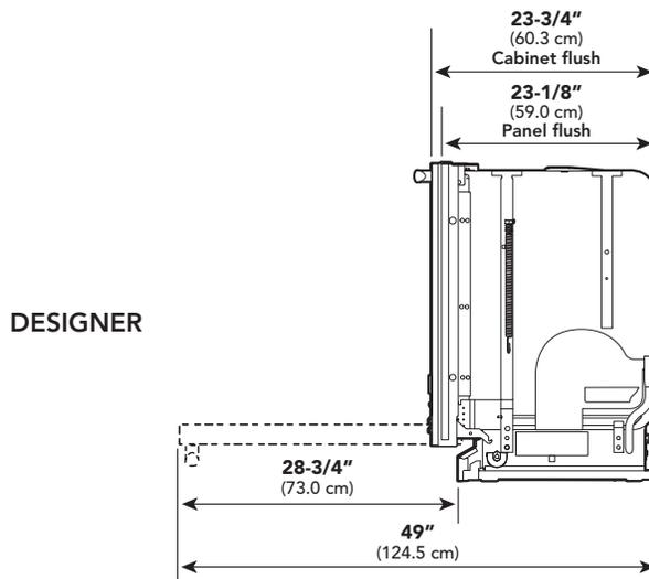
**Note:** If the dishwasher is installed in a corner, there must be a minimum clearance of 2" (5.1 cm) from the side wall so the door can open.
