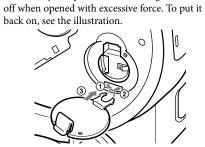
hole in the unit. **2** Insert the right hook into the right hole.
