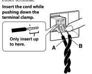
**4** Make sure the AM loop antenna is connected firmly by pulling softly.
