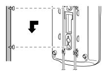
Press and lift out the handset holder, rotate it 180°, then snap it back into place so it holds the handset.
