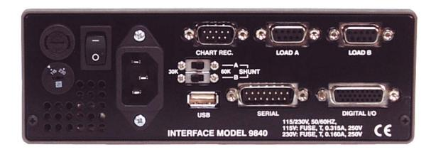
Next connect a load or torque cell to the 9 pin female connector labeled "Load A". You should use the cabling supplied with your Model 9840 and Interface load or torque cell. If you do not have a factory supplied cable see Appendix B for the recommended cell connection.
