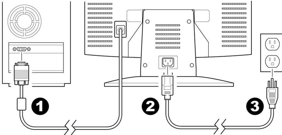
1. Connect the built-in video cable into the 15-pin connector on the back of your computer and tighten the two screws.
