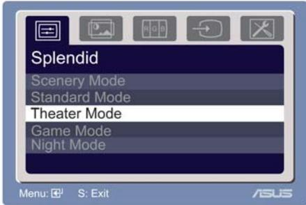
2. Touch **+ / ▲** and **- / ▼** to navigate through the functions. Highlight and activate the desired function by touching the **MENU** sensor. If the function selected has a sub-menu, touch **+ / ▲** and **- / ▼** again to navigate through the sub-menu functions. Highlight and activate the desired sub-menu function by touching the **MENU** sensor.
