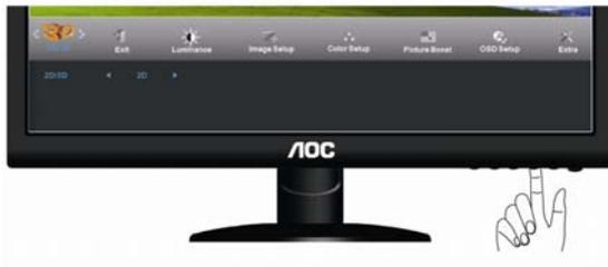
2. HDMI input mode under 2D: Press the Menu key to enter the OSD menu and select the 2D/3D/ menu. Auto (2D), 3D (SBS) and 3D (T/B) modes are available for switchover.
