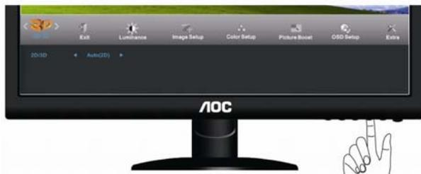
3. HDMI input mode under 3D: Press the Menu key to enter the OSD menu and select the 2D/3D/ menu. Auto (3D), 3D (SBS) and 3D (T/B) modes are available for switchover.
