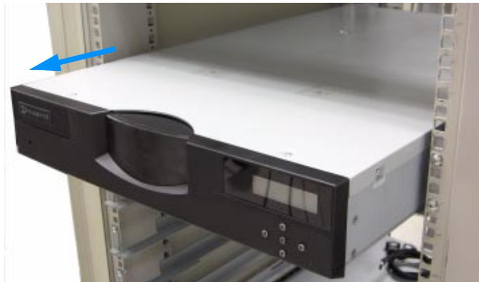
**Figure 9-2** Removing the autoloader from the rack
