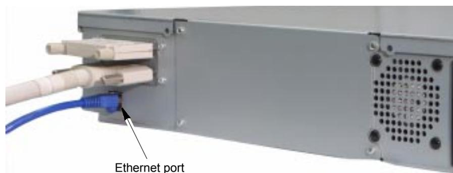
**Figure 2-10** Connecting the autoloader to an Ethernet network
