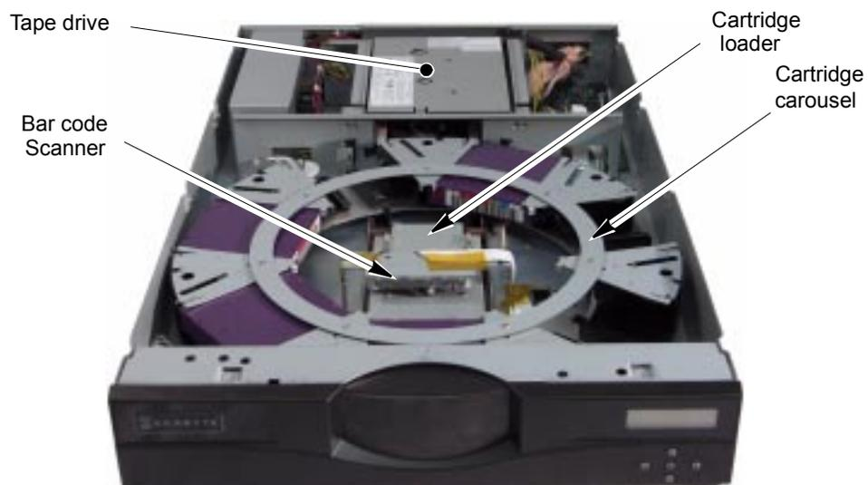
**Figure 1-3** Magnum 1x7 LTO Autoloader internal components
