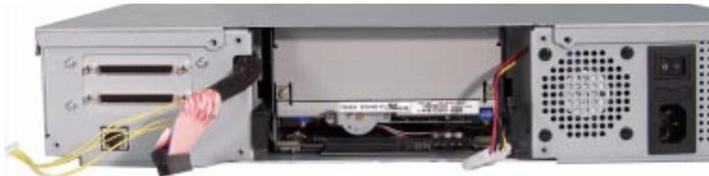
*Figure 7-11 Full height tape drive installation*
