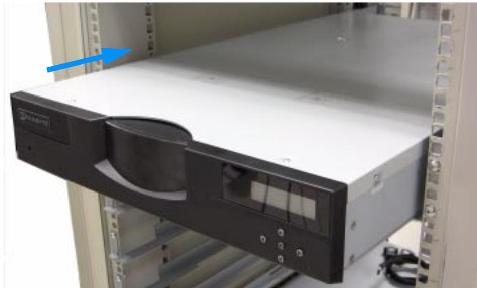
**Figure 2-6** Placing the autoloader on the rails
