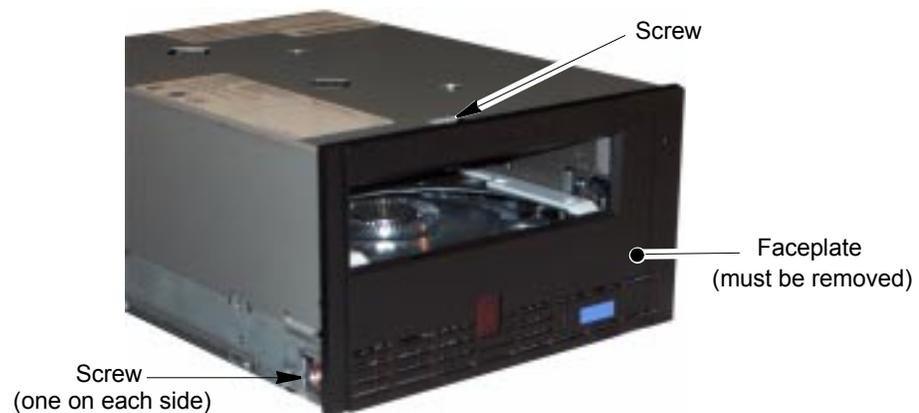
**Figure 7-6** LTO full height tape drive with faceplate
