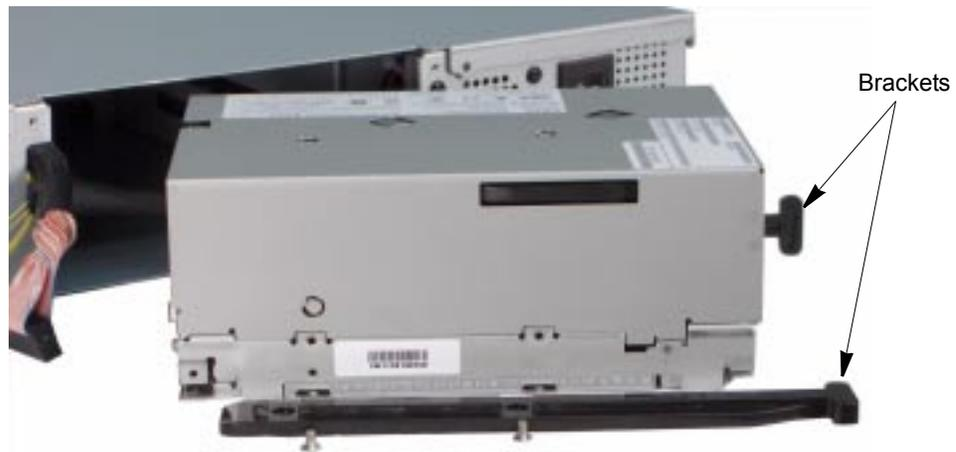
**Figure 7-5** Removing the brackets from the tape drive
