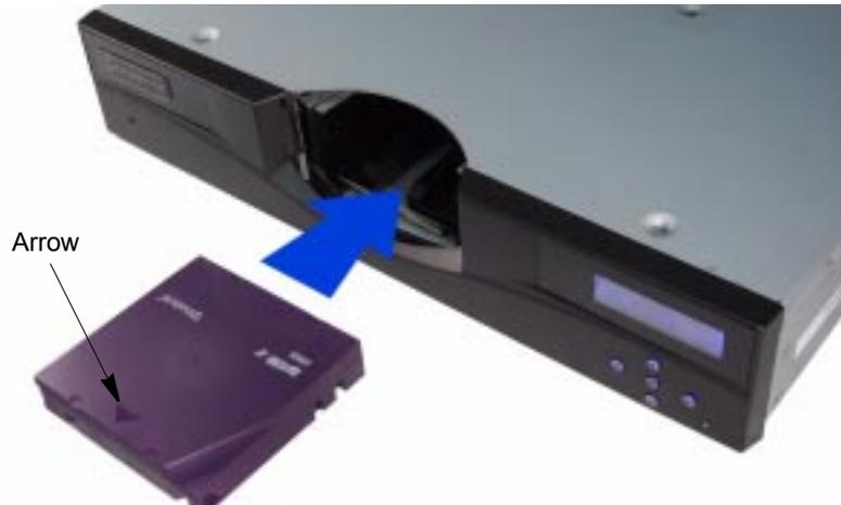
**Figure 5-4** Inserting a cartridge into the autoloader
