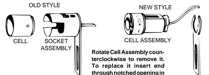
Rotate Cell Assembly counterclockwise to remove it. To replace it insert end through notched opening in bracket and rotate clockwise. NOTE: If bracket is ever removed from burner, Cell Assembly will not fit if bracket is reinstalled backwards.
