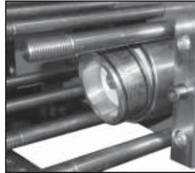
8) Take out the seal case (38) from the valve (if necessary secure 2 screwdrivers in the front O-ring groove to extract seal casing from valve casing). Coat seals with silicon grease before installing.
