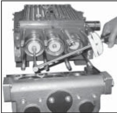
8) Coat the seal sleeve lightly with anti-corrosive grease (e.g. molycote no. Cu-7439) in its fitted area towards the crankcase. Insert the seal sleeves in to their crankcase fittings. Coat the threads of the tension screw (36C) lightly with thread glue and insert it together with a new copper ring (36D) through the ceramic pipe. Turn the pump per hand until the plunger (25) rests against the plunger pipe. Tighten the tension screw at 30 Ft.-lbs.
