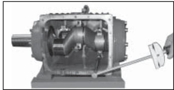
12) Push connecting rod halves together with the crosshead as far as possible into the crosshead guide. Take out bearing cover (14/14A) and push out crankshaft taking particular care that the con rod doesn't get bent. Check surfaces on the connecting rods (24), crankshaft (22) and crossheads (25). Check the surfaces of the crosshead guides in the crankcase for any unevenness.
