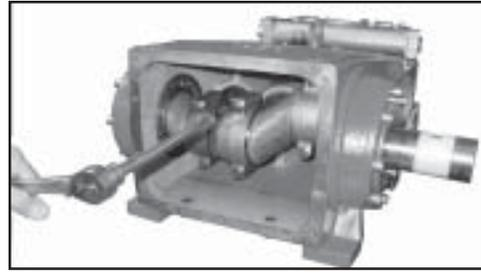
10) Take out plungers and seal sleeves as described above. Drain the oil by taking off the plug (12). After removing the clip ring (33B), lever out the seal retainer (33) with a screwdriver. Open hose adaptor (K11) and remove gear cover (K3). Remove the cooling vane plate (K1) by removing the screws (K4)
