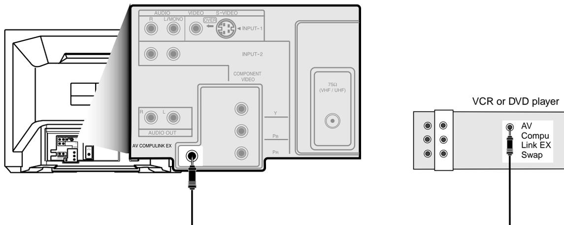
**To Connect:** Plug one end of the AV Compu Link cable into the AV Compu Link EX input on your VCR, DVD, or other Compu Link device. Plug the other end of the AV Compu Link EX cable into the AV Compu Link input at the rear of the television.
