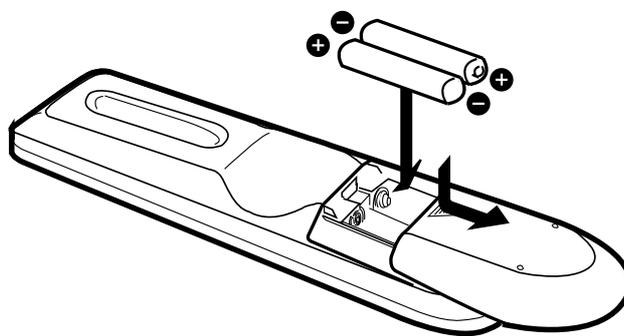
Slide the cover on the back of the remote down towards the bottom of the remote control. Insert two batteries carefully noting the "+" and "-" markings, placing the "-" end in the unit first. Slide the cover back into place.
