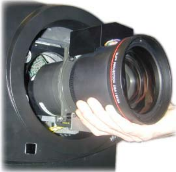
Image 1-3 Take the lens out of the lens block
