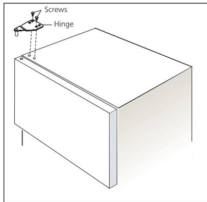
Align doors so there is a parallel gap between doors. Original shipping block may be used to align doors. Adjust doors to cabinet so gaskets seal but do not bind. Tighten upper and lower hinge screws.
