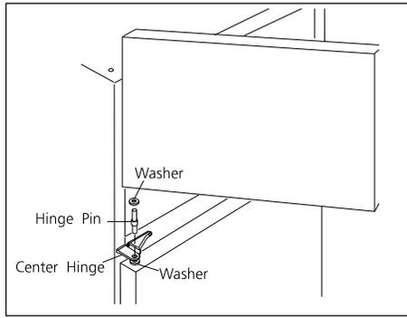
12. Remove plug from upper bearing of door and reinstall on opposite side.
