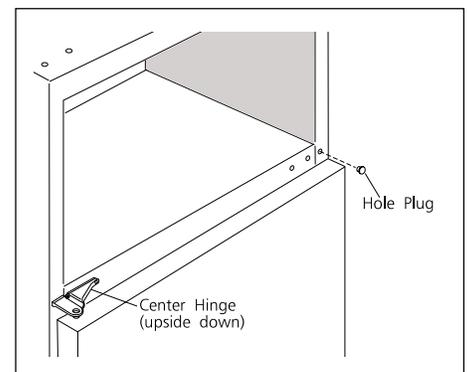
11. Place original washer (some models) over hole in refrigerator door and line up hole in center hinge. Insert hinge pin through both holes. Place washer (some models) on hinge pin, then position freezer door on center hinge.
