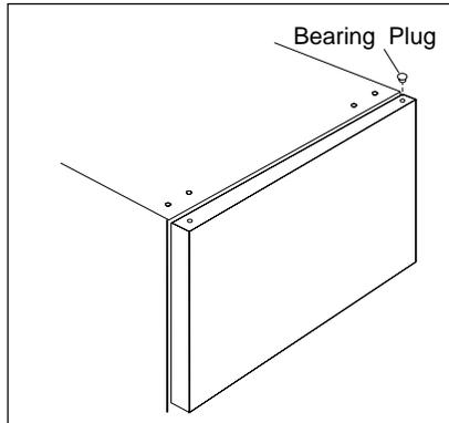
13. Assemble upper hinge to top of cabinet and door. Use opposite set of holes. Do not completely tighten screws.
