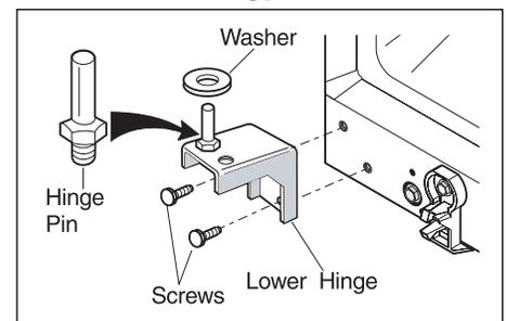
**10.** Turn center hinge upside down and secure to cabinet as shown, using the screws which are in the new holes. Install refrigerator door on lower hinge pin. Align door with edge of cabinet. Hold the door on front of cabinet.
