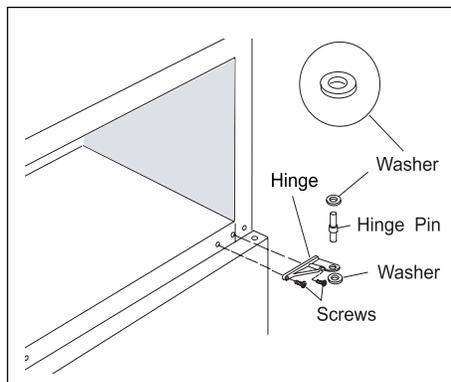
off the lower hinge. Remove the two screws attaching the center hinge. The third outermost screw under the center hinge should be left in place. **Save hinge, pin, and washers (some models) for reassembly later.** Reinstall screws in original holes.
