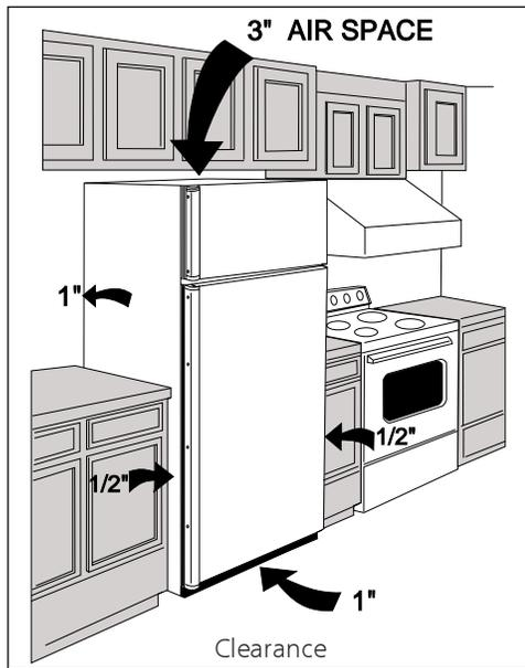
Proper air circulation and leveling will ensure efficient operation.
