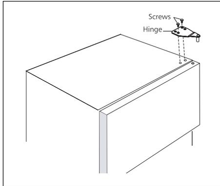
2. Open the freezer door enough to allow it to be lifted off the center hinge.
