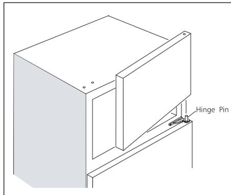
3. With the refrigerator door closed, remove center hinge pin. (Note the arrangement of the upper and lower washers (some models) on the hinge pin. The washers must be reassembled later in the same manner.) Open refrigerator door enough to allow door to be lifted
