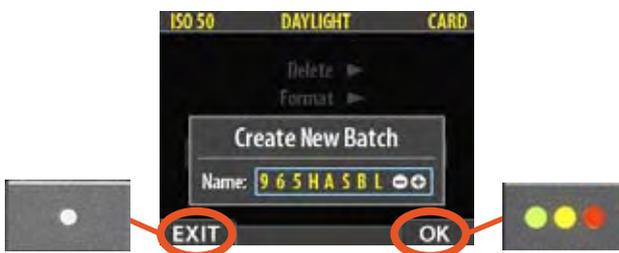
In the next example on the left, the name of a new batch is changed by pressing a combination of the Zoom-in /Zoom-out /SELECTION buttons as well as the navigation button. You can then confirm your choice with the OK (Approve) button or revert to the previous status by pressing the EXIT/MENU button.
