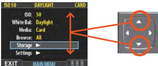
After pressing the MENU button, the main menu list appears. The blue frame highlights where you are on the menu. Press on the 'up' and 'down' symbols on the navigation button to move up and down the list.
