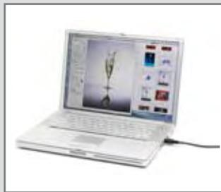
To use an Imagebank with a CF digital back, simply assemble it as described in its manual and connect the two with a standard FireWire 800 (IEEE 1394b) cable. See the Imagebank manual for complete details.
