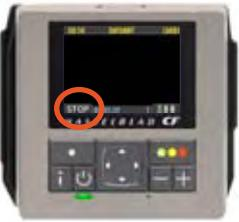
19. Note that the MENU/EXIT button now displays STOP. The sequence can be stopped at any time by pressing this button and the standard menu display returns.
