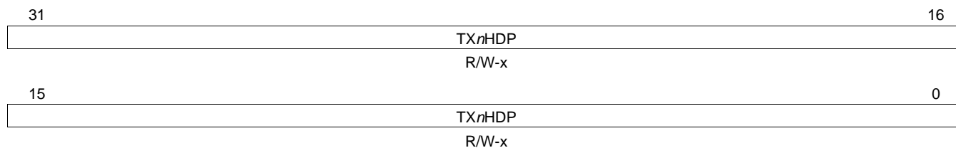
Figure 74. Transmit Channel n DMA Head Descriptor Pointer Register (TXnHDP)
