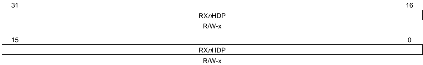
Figure 75. Receive Channel n DMA Head Descriptor Pointer Register (RXnHDP)
